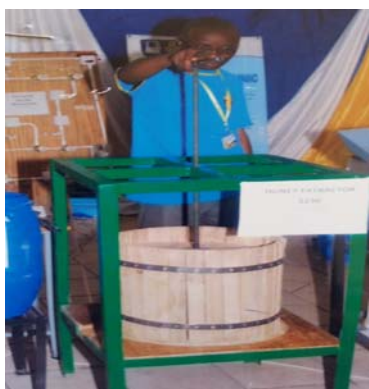
Figure 2: A Honey extractor: A technology that can be used for the extraction of honey. It is made up of a wooden chamber, a lid that can be compressed and a supporting metal structure. It costs $150 and is being sold by the Kwekwe Poly Technic College.
